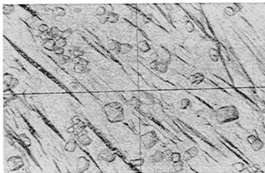
Fig. 14. Photomicrographs of Q-68 (left) and Q-75 (right). (Parallel nicols, \times 100 ) Grain: corundum, Matrix: mullite
